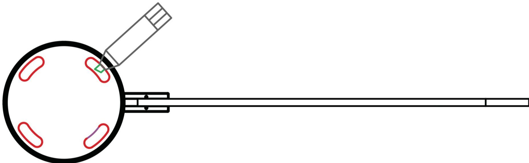
Move the device away and embed M12 \* 100 expansion screws according to the marked hole positions.
